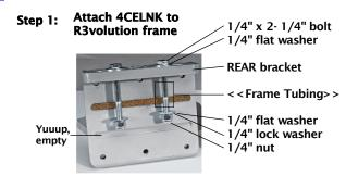
Position so the cork pad is tight against the rail, and tighten the bolts very firmly in place. Don't overtighten, though.
